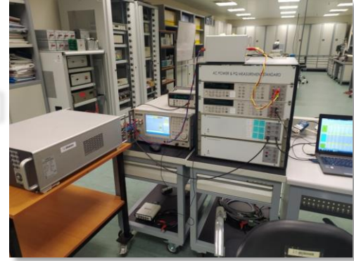
Figure2. Calibration COM 3003 ZERA by using DSWM
